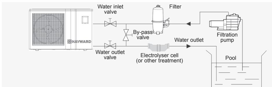
Note: The swimming pool heat pump unit is sold without any treatment or filtration equipment. The components shown on the diagram are parts to be supplied by the installation engineer.
