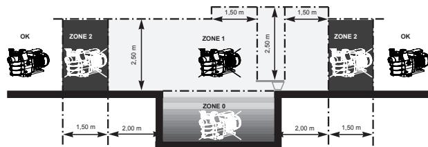
Install the pump in a ventilated and dry place. The motor requires air to flow freely around it to provide for natural ventilation. The pump has to be installed, so that the plug and the wall socket outlet is easily visible and accessible.
