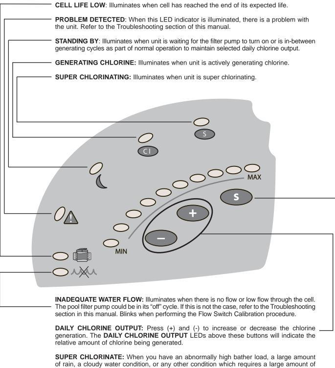
of rain, a cloudy water condition, or any other condition which requires a large amount of purification to be introduced, press the <u>s</u> button. This electronically "**super chlorinates**" (boosts chlorine generation output) the water for 24 hours (filter pump must be on during this time). To cancel super chlorinating, press the <u>s</u> button again.
