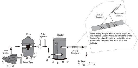
Remove the Template, cut the pipe and install the Nut Assemblies as shown below. Use the included 50 mm Nut Assembly for 50 mm pipe. Place Nut Assembly on each side of the cut pipe (threads face in). Be sure to place the Nut, Compression Ring and Collar on the pipe as shown in the diagram (n°1).
