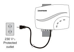
After being powered on for the first time, the PowerSalt will run a diagnostic routine which can take up to 30 seconds. During this time, various LEDs will turn on and off. When finished, the PowerSalt will display a blinking  $\sim \sim \sim$  LED and a solid (LED. Keep the PowerSalt powered for the remainder of this procedure and go to Step 3.
