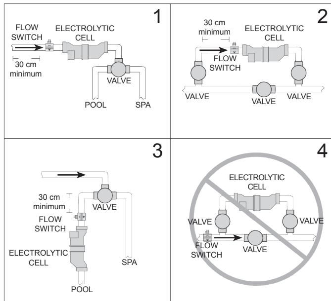
**Flow Switch:** **IMPORTANT:** There must be at least a 30 cm straight pipe run before (upstream) the flow switch. The flow switch must be plumbed before the cell. To ensure proper operation, verify that the arrow on the flow switch (located on top of gray hex) points in the direction of water flow. Refer to the diagram below.
