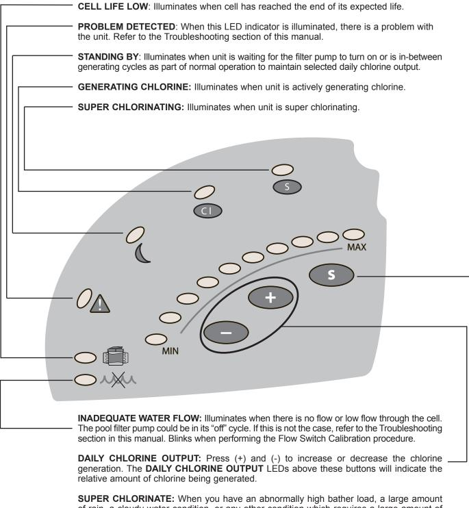
**SUPER CHLORINATE:** When you have an abnormally high bather load, a large amount of rain, a cloudy water condition, or any other condition which requires a large amount of purification to be introduced, press the <u>s</u> button. This electronically "**super chlorinates**" (boosts chlorine generation output) the water for 24 hours (filter pump must be on during this time). To cancel super chlorinating, press the <u>s</u> button again.
