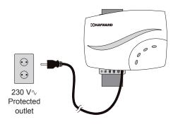
After being powered on for the first time, the Salt & Swim will run a diagnostic routine which can take up to 30 seconds. During this time, various LEDs will turn on and off. When finished, the Salt & Swim will display a blinking AXA LED and a solid ( LED. Keep the Salt & Swim powered for the remainder of this procedure and go to Step 3.
